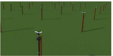
Note: The G-Set Post (above) is not to scale. G-Set Post is generally installed on 2.5" MD ring-main pipe.
