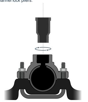
Hand start the NAAN 5022 sprinkler (careful not to cross thread), then finish tightening with a 13/16" open ended wrench or channel lock pliers.
