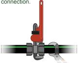
When connecting 2 lengths of tubing, be sure to keep the green lines on the tubing facing up
