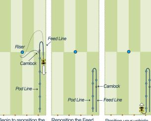
Reposition the Feed Line to run parallel to the pod line (on the far side of the field). The cam fitting that connects to the riser should be near the hook cap.
