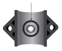
Push the K-Line tapping saddle down over the threaded posts and be certain that the nipple on the underside of the tapping saddle is inserted into the 9/16" hole.
