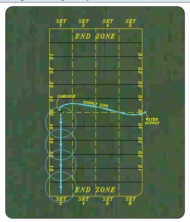
This design can be used for football or soccer fields and consists of a 4 pod system with 8 sets or shifts.
