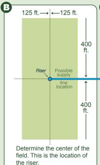
Determine the supply line route from the water supply to the center of the field. The water supply line should be at least 2" or larger from the water source, beginning at a point where sufficient gallons per minute and pressure are available.
