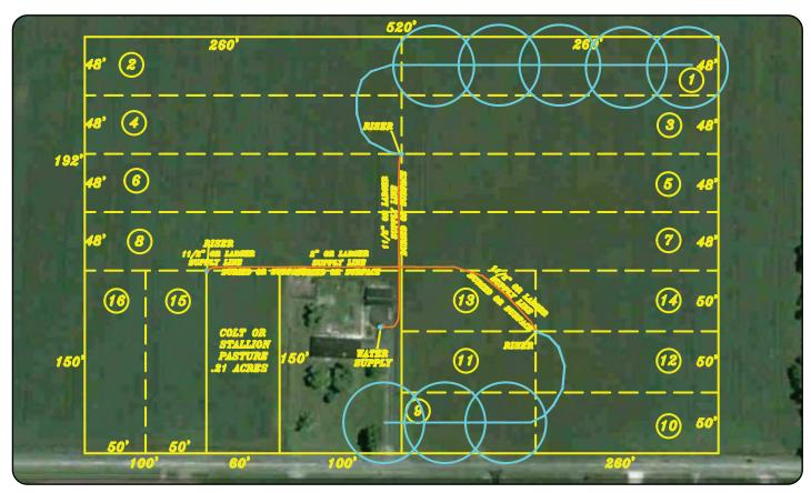
Both K-Line Sprinkler pod lines are operating at the same time
